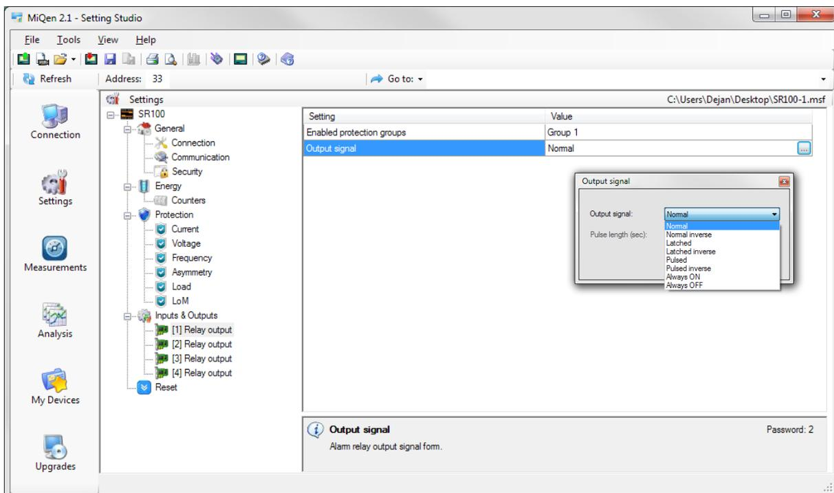
MiQEN Settings overview for Supervision Relay SR100 (example shows relay output module signal options)
