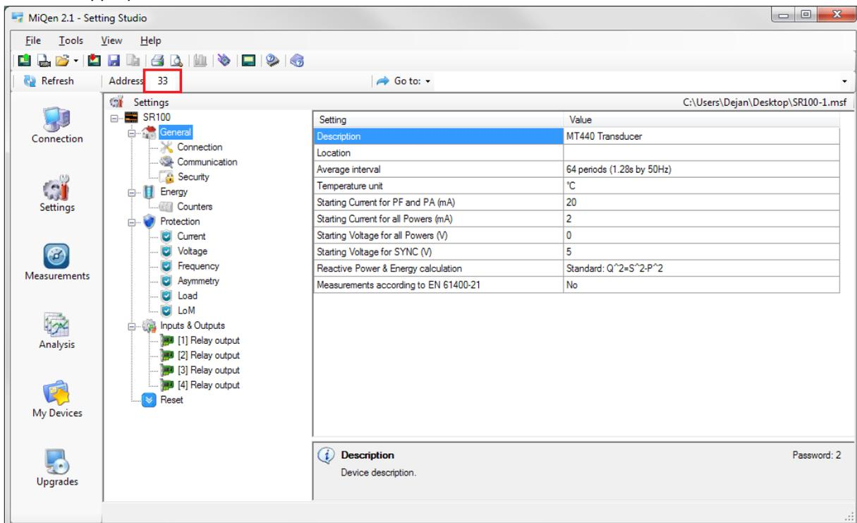
Factory default Modbus address for all devices is 33. If devices are connected in to communication network, all should have the same communication parameters, but each of them should have its own unique address.
