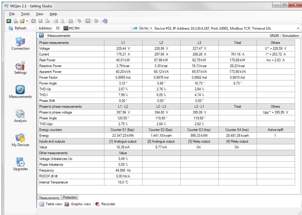
The screenshot shows the 'Measurements' window in the MiQen 2.1 - Setting Studio software. The window title is 'SR100 - Simulation'. The address bar shows 'Address: 33' and 'Device #33, IP Address: 10.120.4.187, Port: 10001, Modbus TCP, Timeout 10s'. The main area displays a table of measurements:
